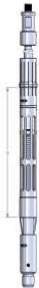
Fig 1. Proper operation of 'ROTD-2' Shifting Tool requires that dimension 'A' be adjusted accurately and the proper Collet be installed prior to running the Tool.
